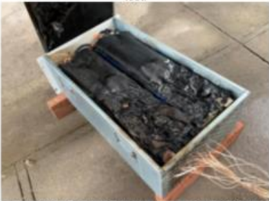
Figure 28d. Photo 03 of initiating module M20 after test.
