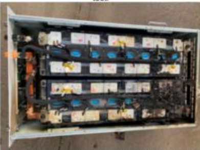
Figure 28f. Photo 05 of initiating module M20 after test.
